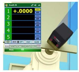
3. Rotate the A-Axis 180 degrees. In this case, the reading is -.0011, which means the A rotation axis is tilting forward relative to the Y-Axis by .0011 in 18 inches.
