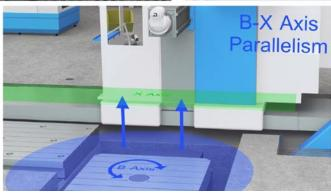
1. To check the B rotation, move the target to one of the corners of the table. Zero the display and then rotate the table 90 degrees.
