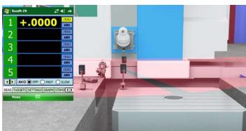
2. The display shows +.0024, indicating that the table rose by .0024 as it rotated. Therefore, the rotation plane is sloping up from left to right relative to the main table (recall that the main table was the reference for the horizontal red laser plane).
