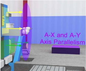
1. To measure the A rotation, we'll use the gold laser plane and a target mounted on the spindle. For both the A-Axis and the Tram measurements, a simple tram bar can be inserted into the spindle with a target attached.
