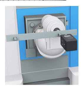
2. Adjust the ram and zero the target.
