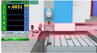
5. Plane5 analyzed the data and found that the flatness of rotation is .0010" TIR and the parallelism to X is .0011 in./ft. and .0002 in./ft. to Z.
