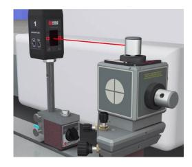
4. Turn on the laser rotation (which also turns on the targets). Target #1 data displays in the Read9 software on the PDA. Zero the display. Remove Target #1 and replace it with Target #2. Zero the Read9 display for Target #2. Repeat the process for Target #3.
