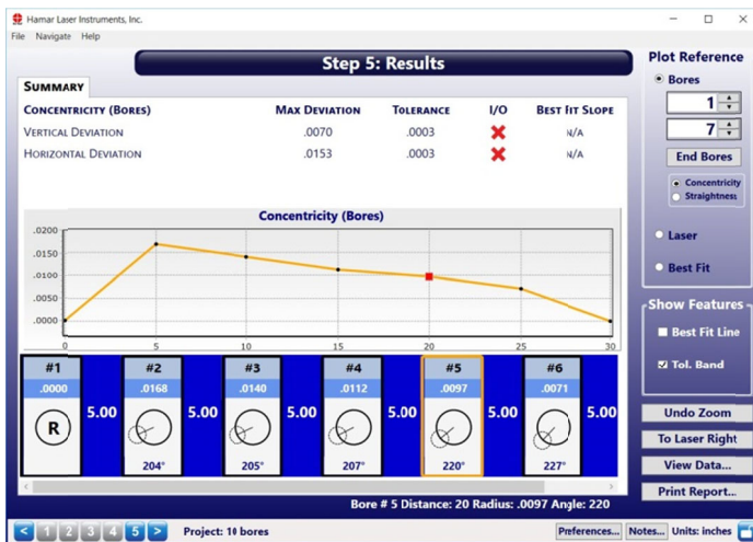
Bore9 – Step 5: Results – Concentricity Plot using the End Bores as a reference.
