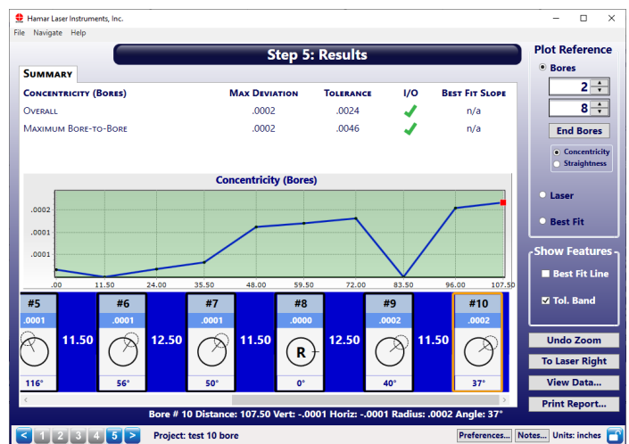
Bore9 – Step 5: Results – Concentricity Plot using Bores 2 & 8 as a reference.
