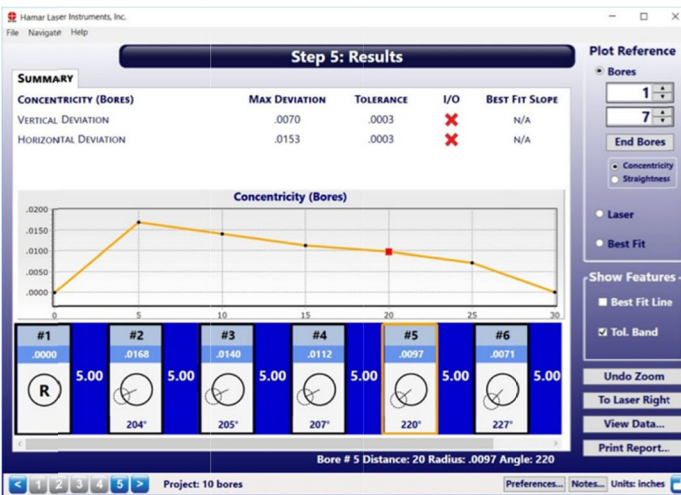
Bore9 – Step 5: Results – Concentricity Plot using the End Bores as a reference.
