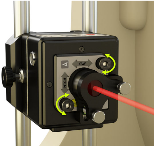
Adjusting the H & V angles on the L-703B to center it at the far bore
