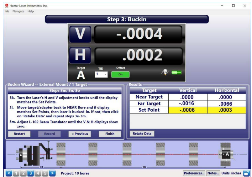
Bore9 - Step 3: Laser Steered to Zero (Bucked-In)
