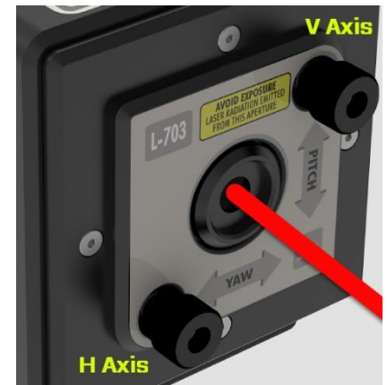
Figure 4 - L-703S Laser showing Pitch & Yaw Adjustments
