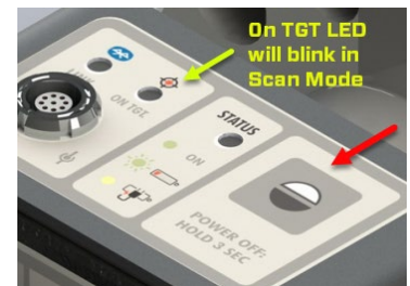
Figure 8 - T-1295/1296 Control Panel
