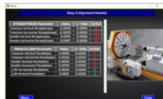
Lathe10 - Step 3 Alignment Results
