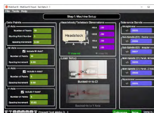
Lathe10 - Step 1 Dimensions and Tolerances
