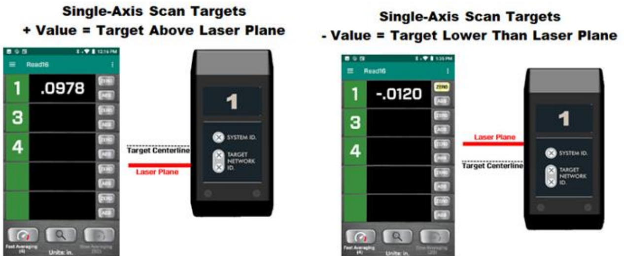
Figure 10 – Single-axis Scan Target displaying positive (+) and negative (-) values
