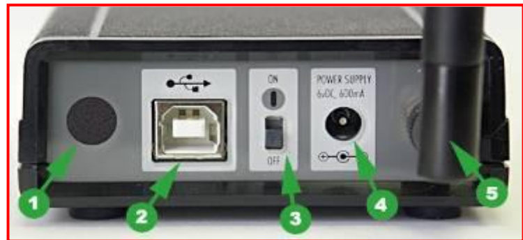
Figure 19 – The A-910 Radio Transceiver/Hub REAR PANEL
