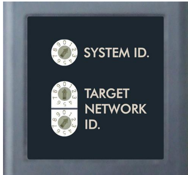
Figure 13 – Unitarget ID Switch set to 1
