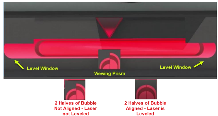
Figure 15 –L-740SP Split-Prism Level Vial Assembly for L-740 Series Lasers
