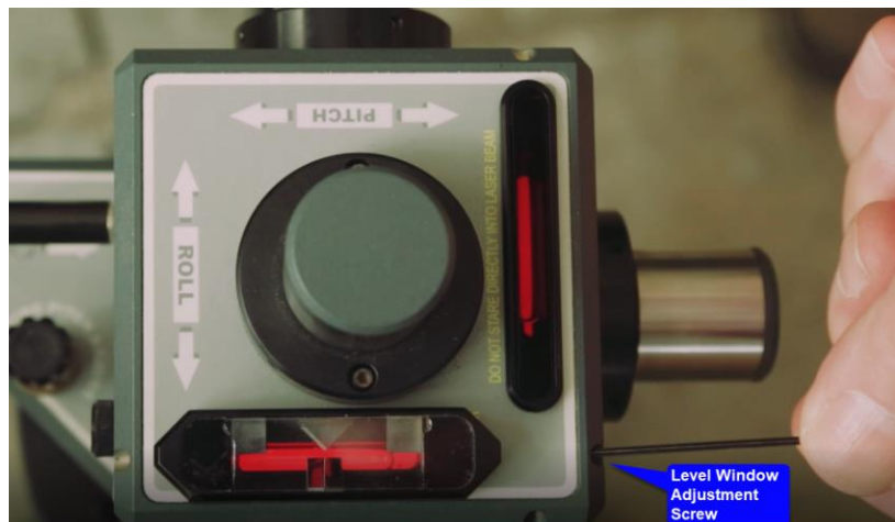
Figure 19 – L-733 (top view) showing location of Precision Level Vials and corresponding adjustment screws. Also see our YouTube video: How to Calibrate Level Vials .
