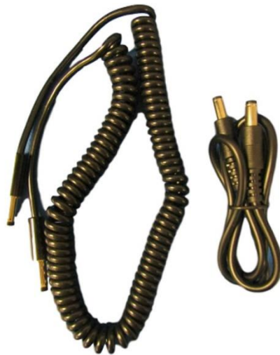
Figure 5 - Cables to connect unit to Output on laser.
