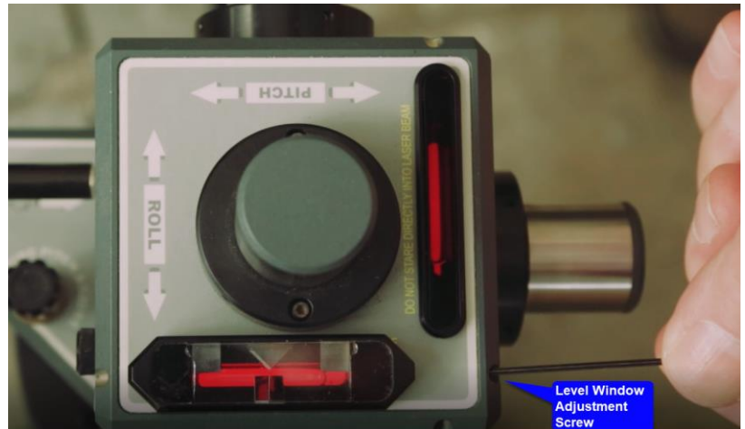
Figure 18 – L-733 (top view) showing location of Precision Level Vials and corresponding adjustment screws. Also see our YouTube video: How to Calibrate Level Vials .
