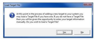
4. If you clicked **No, enter the required information:** Target Name, Calibration Date, Target Network ID, (see *Setting the Target System ID and Target Network ID* on Page **58**) and depending on your target, the Calibration Constants. The Serial Number, Focal Length and Description are optional. Note that the **Name** field can contain *any* name that will readily identify the target.
