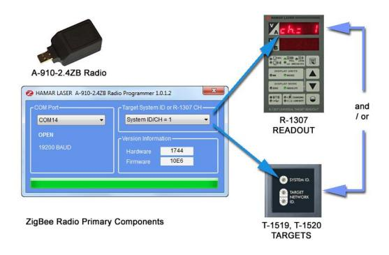
Figure 7 – Setting the Targets/Readout to the same System ID and Channel
