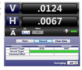
4. Rotate **Target A** to the normal position. Click **Record** for the **Target A** data box. This automatically calculates a display offset that is applied to raw values for **Target A**.
