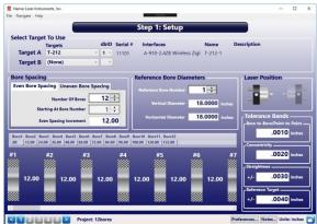
3. Record readings in both the *Normal* and *Inverted* positions for each bore location (number). The user can take all of the *Normal* readings (select *Normal Only* in **Auto Step**) and then all of the *Inverted* readings (select *Inverted Only* in **Auto Step**) or take *Normal + Inverted* readings at each location (select *Normal and Inverted* in **Auto Step**).
