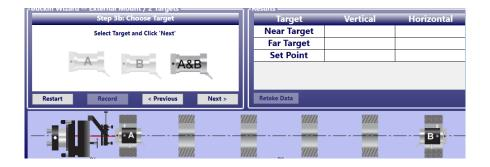
10. Enter the distance from the laser pivot to the Near Target and the distance from the Near Target to the Far Target (see graphic at the bottom screen to see how to measure the dimensions – shown here). Click **Next**.
