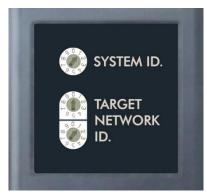
There are three rotary DIP switches located on the right side of the target, shown in Figure 29:
