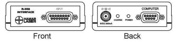
Figure 2 – R-358 Computer Interface Connections
