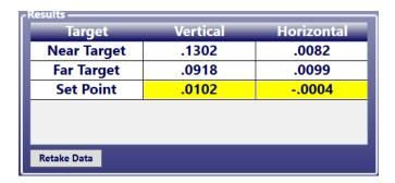
7. Follow the on-screen instructions to steer the laser beam so that the V and H displays match the V and H **Set Points.**
