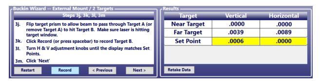
14. Adjust the H and V knobs on the L-706/L-708 until the **Target B** display values equal the **Set Points.**
