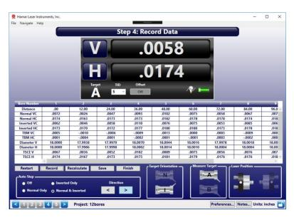
4. During the data recording you will notice that the Diameter V and H rows will show the word "Processing". This is normal. The diameters will not be calculated until all the data has been taken. When the last data point has been taken, the calculated diameters will appear in their respective rows. This data will also appear in the data grid in the report and can also be viewed by clicking **View Data** in **Step 5**, which brings up the data table from the report.
