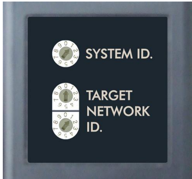
Figure 6 – Unitarget ID Switch set to 1
