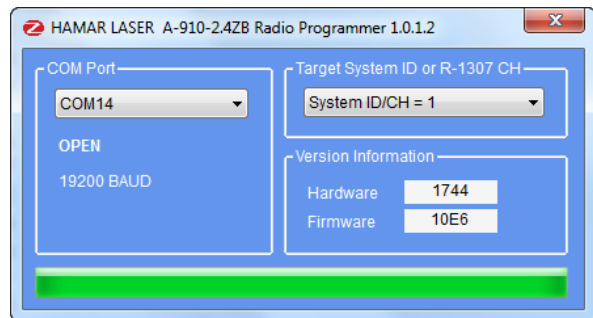
Figure 3 – A-910 Utility showing the COM Port, System ID and Channel settings
