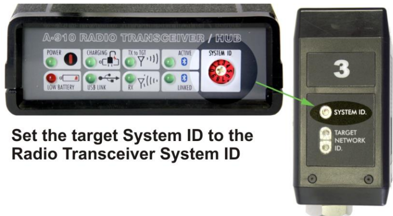
Figure 8 – Radio Transceiver and Target System ID
