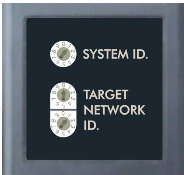
Figure 10 – Unitarget ID Switch set to 1
