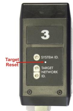
Figure 2 – Reset hole for target
