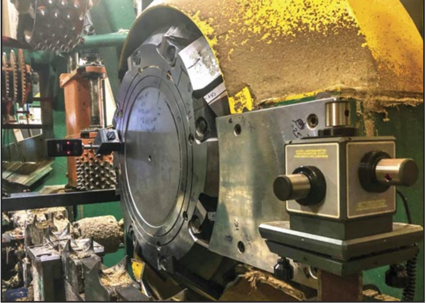
Aligning canter heads and anvils for lead, plumb and offset using the L-743 triple scan laser and A-1519-2.4ZB Wireless Targets. Below, at left, aligning track and rolls of secondary breakdown line; right, aligning bed and press rolls parallel and level on secondary breakdown
