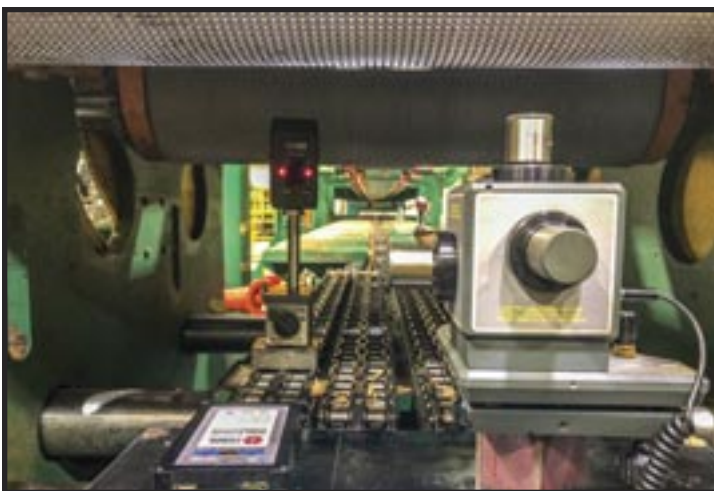
Aligning canter heads and anvils for lead, plumb and offset using the L-743 triple scan laser and A-1519-2.4ZB Wireless Targets. Below, at left, aligning track and rolls of secondary breakdown line; right, aligning bed and press rolls parallel and level on secondary breakdown
